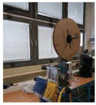
Materials and parts used for production of cable harnesses depend on the specification, intended use of the customer and its request. Wires can be printed along their entire length with the possibility of different label or its orientation. Cable harnesses are processed on the balancing tables with templates. This ensures accurate shaping of individual branches of cable harnesses for their use in electrical devices and vehicles.
